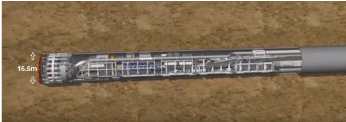
Plate 3.1 Cutaway view of a large diameter tunnel boring machine (Herrenknecht)
