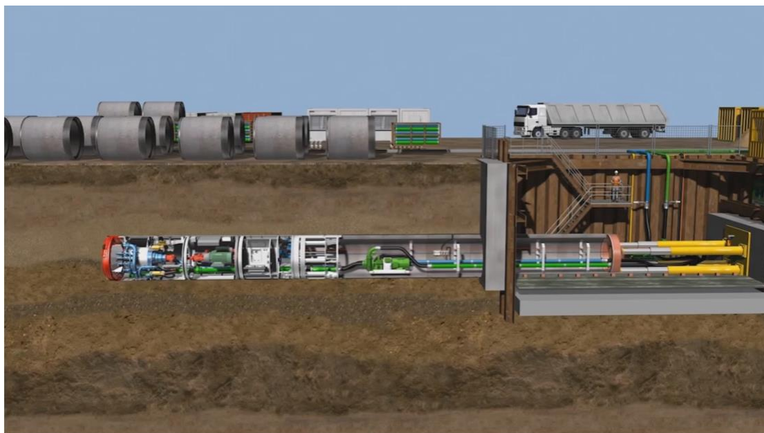
Plate 3.2 Cutaway view of a micro tunnel boring machine and pipejacking system (Herrenknecht AVN)
